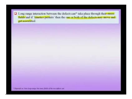
The association of defects can take place, through the long range stress fields associated with these and if kinetic permits, then one or both of these defects may move and get associated. Now, that means that if these defects originally existed in isolated form and it is get interacting actually through a long range stress field. Like an example of one dislocation to another dislocation, then they actually attract each other.
