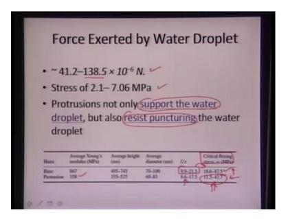
And the force exerted by the water droplet it comes out to be around 41.2 to 138.5 into 10 power minus 6 Newton, which corresponds to a stress of around 2.1 to 7.06. And there are two very key features out here that protrusions are not only supporting the water droplet, but they are also resisting the puncturing of the water droplet.
