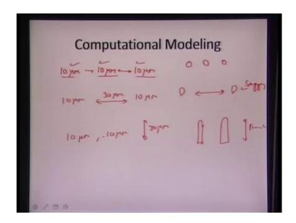
And we see that we have maintained three kind of roughness, in one case we utilized 10 micro meter diameter which is being separated by 10 micro meter of distance and all these pillars are something like 10 micro meter in height. So, we have 10 micron, 10 micron, 10 micron out here, droplet size of around 10 microns again 10 microns of pillars 10 microns meters apart.
