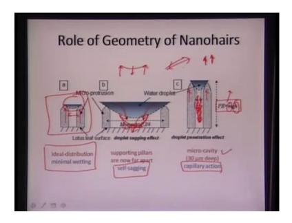
So, how do they really govern the overall wetting? In this case, we see a particular lotus leaf surface these are all the protrusions micro protrusions and once they are certain distance apart around 10 microns, it shows a regular support of the water droplet. And this is the ideal distribution leading to the wetting, but once we start separating the pillars by a distance, we start seeing that the water droplet will tend to sag, and the sagging effect will lead to the wetting of the surface.
