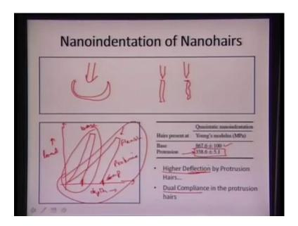
And coming to the nano indentation of nano hairs, if we indent a particular surface all these nano hair will form will buckle. So, if we had this particular nano hair and if we tend to indent it using a nano indenter, this one will basically buckle and from the low, from the low depth curve, we can say which one has a higher ((Refer Time: 28:47)) modulus.
