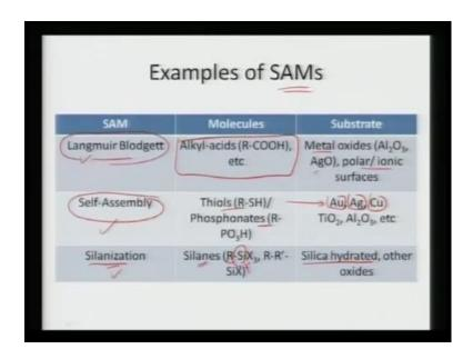
So, we can see examples of self assembled monolayer's, so we have Langmuir Blodgett, it generalize very prominent on the alkyl acids such as RCOH, it is predominant on metal oxide or polar or ionic surfaces, whereas thiols are self assembly. Self assembly retreated by thiol phrosphonates it has high affinity for materials such gold silver copper and so on and third is the Stalinization.
