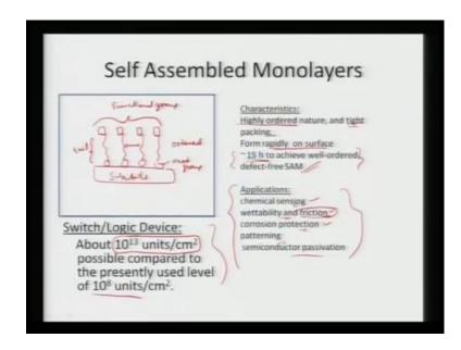
So, seeing that self assembled monolayer's first of all they have highly ordered structures they are nature is highly ordered and it provides very tight packing and it forms very rapidly on the surface. To attain a particular order, it that is the time consuming step or that is the step decide the rate deciding step.
