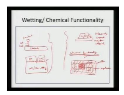
So, we can see first of all we have a head group which is lying on a substrate, so we have a substrate, then we have a head group with certain tail and then a functional group. So, we have head this is a tail, this is also called as spacer, so depending on the length of this tail, we can somehow control the how this structure will come out to be, so in one case we can make the surface highly wetting or non wetting.
