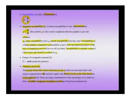
The other important quantity in the field of magnetism are the magnetic field strength h, the magnetization m, the magnetic flux density B, the susceptibly chi which we said the very important material parameter which will discusses in detail later, and the permeability mu. And apart from this, we also talk about the magnetic anisotropy. So, these are the important quantities in magnetism.
