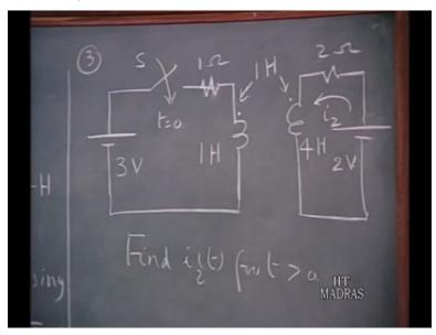
Now, the third example, is concerns use the transform diagram approach where mutual inductance. So, you have a 3 volts source connected to a series circuit of 1 Ohm and the primary coil having a self inductance of 1 Henry. It is couple to a secondary coil of 4 Henry self inductance the mutual inductance of 1 Henry, this is the mutual inductance.
