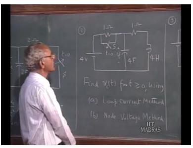
Second problem is this: in which we have a 2 loop circuit consisting of an inductor and a capacitance so on. The switch is kept close for a very long time that enables you to find out the initial condition respect to the capacitor as well as the inductor. And you use them the transform diagram it 4 volts 1 Ohm, 4 Ferrates, 1 Ohm, 4 Henries.
