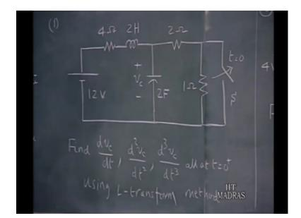
First problem. So, in this problem you are having a 12 volts vc source connected to circuit consisting of a 4 Ohms resister 2 Henry inductor 2 Farads capacitor in shunt and the 2 Ohm resister and a 1 Ohm resister. Now, this switch s is kept closed for a very long time since, steady state is reached and then it is opened t equals 0.
