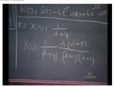
Now, response to e to the power of 4 t ut. So, x of s the input is e to the power of minus 4 t this is 1 over s plus 4. So, y of s corresponding to this is 1 over s plus 4; that is x of s times h of s h of s is s times s plus 5 divided by s plus 1 times s plus 2; that is the y of s. So, you make the partial fraction expansion of that.
