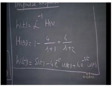
Impulse response, h of t is the Inverse Laplace transform of h of s this is h of s. So, h of can be expanded by means of partial fraction expansion so, it will turn out to be 1 minus 4 over s plus 1 plus 6 over s plus 2. So, if this rational function makes the partial fraction expansion of the rational fraction you get this because the numerator and denominator as the same degree polynomial s square divided by.
