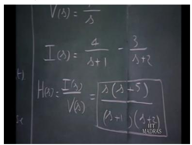
Therefore, the input Laplace transform is 1 volt. So 1 volt is given t equals 0 to this network therefore, it is a step function really v of s is 1 over s the current in the network as the Laplace transform of this 4 up on s plus 1 minus 3 up on s plus 2 4 up on s plus 1 minus 3 up on s plus 2 that is the expression for the current.
