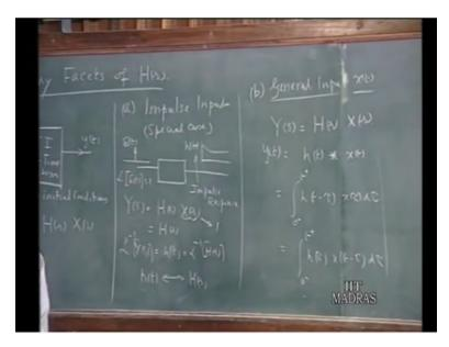
Now, using this information general solution in time domain, general input x t, suppose you are having, and you want to find out the output in time domain. We know that y of s equals h of s times x s. Now, by the convolution property, we know if y of s is the product of two quantities h of s and x of s.
