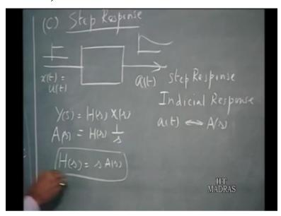
A third aspect; I also mentioned in our earlier discussion that step response is also a way of characterizing a linear system. So, let us see how it is related to a system function h of s. So, in step response we are thinking of unit step applied as a input. So, x t is u t, and the corresponding output whatever you are having here, is given a special symbol a t.
