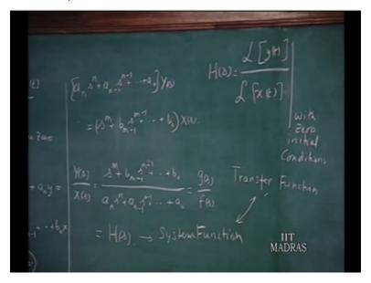
So, that makes the transforming this equation a very simple task. So, if you take the Laplace transform of that, you have a n s to the power of n plus a n minus 1 s to the power of n minus 1 times a not plus a not times n of n equals the Laplace transform of the side of equation, which is n to the power of n minus 1 on up to n not multiply n of n minus 1 on up to n not multiply n of n s.
