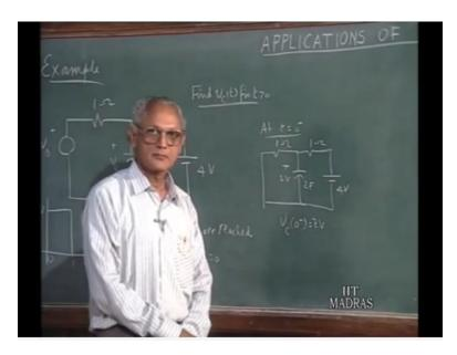
So, to do that let us see the system, the various parameters the system at various variables in the system at t equals 0 minus. At t equals 0 minus this voltage source is 0. You have a 1 ohm resistance, a capacitor, another 1 ohm resistance and a dc source. This is 4 volts, this is 1 ohm, this is 1 ohm, and this is the capacitor of 2 farads.
