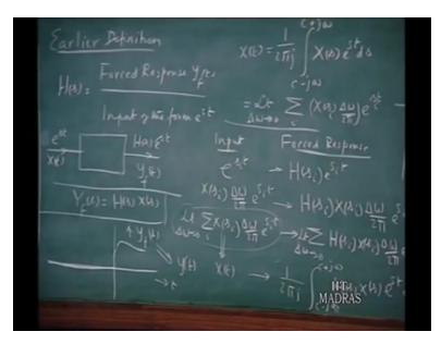
You recall that earlier we said in our introductory lectures that system function is the ratio of the forced response of the system, to the input when the input is an exponential signal. In other words earlier definition was h of s was defined as, the forced response y f of t to an input of the form e to the power of s t.
