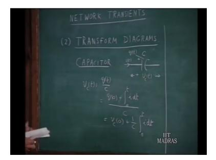
The second approach will take for the analysis of network transients is, what is the called the method of using transform diagrams. Before, we actually illustrate this method. Let us look at some preliminaries. To start with will take the capacitor, we know that the terminal equation is over capacitor can be put in the form, that v c of t is q of t over c. So, if the capacitor here, parameter c, this is v c of t. And the charge and the capacitor, suppose is q of t, the current is i of t.
