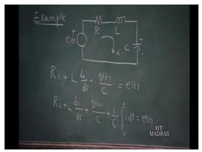
In considering the network transients, we can first form the differential equation pertaining to the network. And then, transform the differential equation in to the Laplace transform domain and arrive at the solution. This is the method that suggest by itself and this is a more fundamental method.
