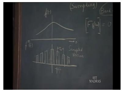
Suppose, we do not consider f of t for the entire time duration, but generate from f of t a sample version of that. That means, this is f of t we have variation; you do not consider the entire variation by take samples from that tiny interval like this. So, we consider f of t for small intervals of duration d and the period between 2 successive samples is t not. This we may call sampled version of f of t we will call that f star of t; this is sampled version.
