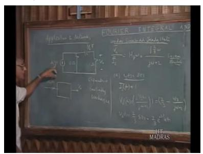
So, let us take an example, to illustrate this suppose, I have a current source I s of t which is given to a circuit like this, where this is 2 Ohm resister 1 by 6 Faradays capacitor and 1 Ohm
