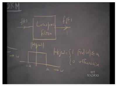
Let us see, how this such a concept can be made use of in practice. Let us assume that, this particular f of t which we had the exponential signal is put through a low pass filter. And we get output signal f 0 of t this low pass filter has a characteristic like this. H of j omega magnitude a low pass filter essentially allows all frequencies up to a certain point then shuts off all other frequency components.
