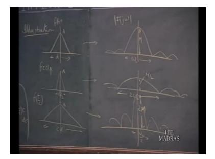
So, this again has got some important aspects in relation to scaling of time functions. Let me illustrate this; illustration of this suppose we had a time which is given like this a and stitching from over an interval d. And let we imagine that its Fourier transform would be like this magnitude spectrum I am plotting and this is equal to let us say some omega I will say some omega 0 whatever it is.
