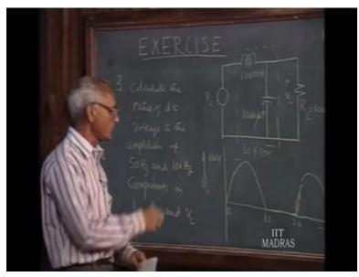
The third example let us consider circuit where we have an input voltage. Which is half wave rectify sine wave like this, with an amplitude of 100 volts this is vi 0, 10, 20 this is t in milliseconds. That means; this 50 cycle's wave from which we generate half wave rectified sine wave 100 volts.
