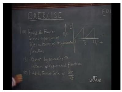
First problem, Consider a wave like this triangular wave; this is the voltage wave v1 of t. So, this is the triangular wave saw tooth wave as it is called with an amplitude e and period t not. Find the Fourier series expansion of v1 of t in terms of trigonometric functions. That is, in terms of a not a n and bn repeat this by expanding f t in terms of exponential functions, that is; in terms of cn c.
