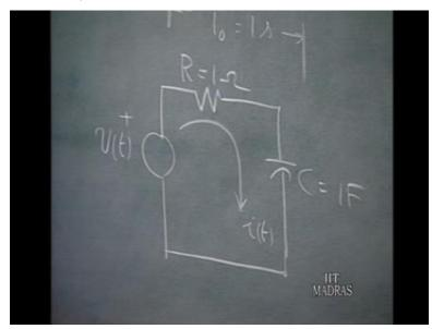
Now, if a voltage adding this type of waveform v of t is given to an rc circuit containing a resistance of 1 ohm and a capacitor of 1 farads. Let under steady state the current i(t)
