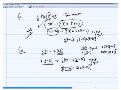
So, let me take another simple example to illustrate how you go about finding time variant or time invariant systems. Here is the other example y of t equals t times x of t. Okay, so, it turns out if the independent variable t appears by itself in the input output equation that's one of the hints to show that it is a time variance system. It is not a time invariant system.
