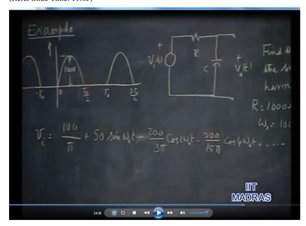
In this example, we will consider that a waveform of a voltage, of this shape, is applied to an R C circuit. And the voltage across the capacitor is taken to be the output voltage. So, we will imagine that the peak value of this half wave rectified, sine wave is 100 volts. Now, this voltage is applied across the R C circuit. And we are interested in finding out, the significant harmonics both the input and the output voltage.
