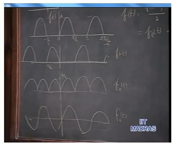
Consider this example, where we are dealing with a f of t, which is a half wave rectified sine wave of amplitude a. And a fundamental period T not. Now, when you look at this, this waveform does not have either an even symmetry or an odd symmetry. You recall that we had observed earlier, that any given function can be split up, as it is even part and odd part respectively.
