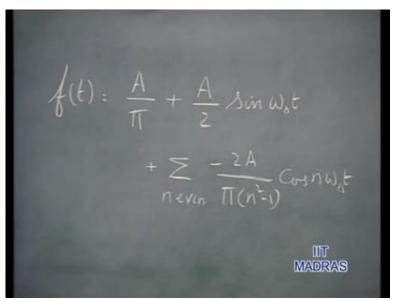
So, the Fourier series for this waveform would be, f of t equals the d c term A upon pi. Plus the fundamental term which comes from the odd part, A upon 2 sine omega not t. Plus the remaining terms in the Fourier series expansion of the even part of the function, which will be minus 2 A over pi times n square minus 1 cos n omega not t. For n even starting from n equals to onwards.
