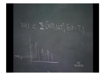
So, x t can be regarded as: approximated as number of impulses. A particular impulse which we have sketched in the figure is x tou y delta tou that is, the area under the curve, that is the magnitude of the impulse and that impulse is situated at tou y. So, this is the impulse that we are talking about.
