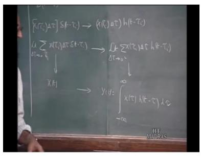
So, tou i is not discrete points. Continuously it exists delta t d tou, that is your y of t. So, y of t is obtained as x tou h t minus tou d tou. That is how we can obtain in the limit, the output y t corresponding to this x of t and in general, the most general case; this integration must last for minus infinity to plus infinity, but in the more usual cases the limits can be further restricted as we will see at a later point of time.
