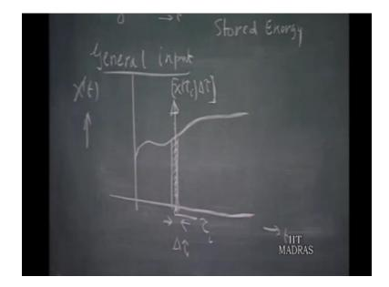
Now, any arbitrary except t given as an input something like this; this is the general input, can always be thought of; suppose, you take a small narrow section of width delta tou and then let this, at the center we will call that tou y. This point tou y and this section of the input; a narrow section of time, this area can be replaced by an equivalent impulse.
