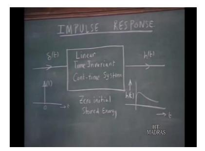
To a unit impulse will give all the information that is needed for us, to find out the response to any arbitrary input. Let us see how we go about it. This is a linear time invariant continuous-time system. It is represented as a box like this. Suppose the input is delta t; a unit impulse at the origin and let the corresponding response h of t is given like this.
