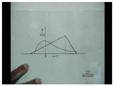
So, for various shifts you find out the product of these 2 curves and find out the area under that curve. And this is how, 1 can calculate the convolution values, integral values for elementary time products. So, the key words here are: fold, shift, multiply and integrate.
