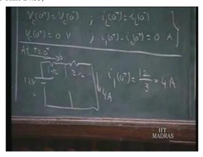
The current in the circuit the current in c here at t equals 0 plus is 4 Amperes. This is 4 Amperes so what does it mean?
