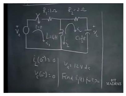
So, let us take an example let us consider this particular circuit to illustrate the differential equation approach. We have an inductor and capacitor in the circuit and the inductor and capacitor provides the initial conditions that are necessary to solve the problem and normally. The initial conditions are given pertaining to a situation before a closure of a switch.
