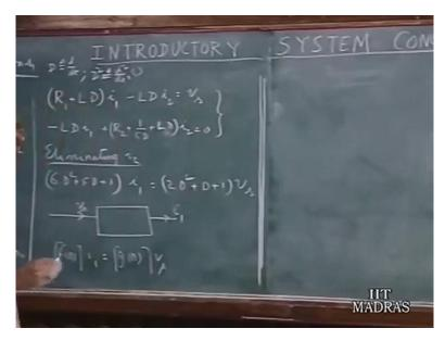
And this can be written as r1 plus ld derivative operator operating on i1 because derivative operator d is equivalent to d i1 by dt. D times i1 is d i1 by dt minus l d operating on i2 equals Vs. That's the first equation where by definition d by definition is d up on dt.
