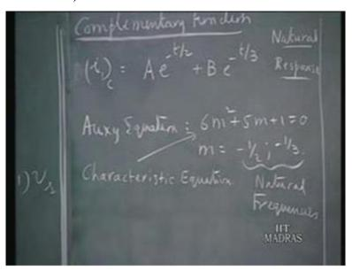
The complimentary function solution this is part of the solution. So, i1 complimentary will consist of 2 terms depending up on the roots of the Auxiliary equations. So, the Auxiliary equation we have here is 6m square plus 5m plus 1 equals 0. This is the 6d square plus 5d plus 1 is 0. We substitute use m for d and this is what we get as Auxiliary equation and the values the solutions for this will be m equals minus half and minus one-third.
