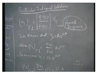
But before we proceed further we need to have the particular integral solution. The particular integration solution from your elementary study of differential equations will be obtained as g of d by f of d operating on the forcing function Vs.
