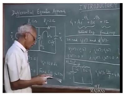
So, the total solution is i1 equals a e to the power of minus t up on 2 plus b e to the power e minus t up on 3 plus 12. This is the natural part natural response this is the forced response. Now, that we have got the total solution the form of the total solution we have to evaluate these arbitrary constants a and b for that we need to know the initial conditions, from the initial conditions you should be able to find out a and b.
