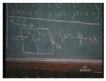
At t equals 0 plus what is the value of the voltage across the inductor. This is equal to VL 0 plus. What is the value of the voltage across the inductor at 0 plus.2 Ohms and a current i1 of 4 Amperes. Therefore, 8 Volts the capacitor voltage is 0 so at t equals 0 plus this is 8 Volts.
