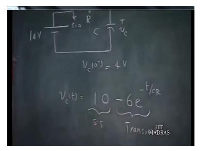
Let me take an example to illustrate this idea suppose I have a 10 Volts. D.C. source connected to a r c circuit with an initial capacitor voltage of 4 Volts and I would like to find out how the capacitor voltage behaves for time t equals 0 onwards if the switch is closed at t equals 0.
