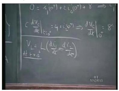
That C dVc dt that is the current in the circuit at t equals 0 plus equals 4. This is i2 0 plus.i2 0 plus is the same as i1 0 plus from this we observe that dVc dt at t equals 0 plus dVc dt 0 plus 4 divided by 2 which is equal to 2C equals half a Ferret, C equals half a Ferret. Therefore, this is equal to 8 Volts per second. Therefore, this substitute dVc dt is equal to 8.
