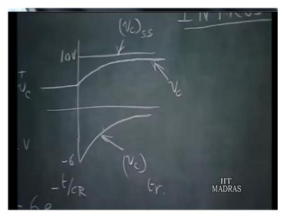
So, the capacitor voltage can be this is 10 Volts, this is d c steady state new steady state of course as 4 Volts and then you have a transient term which has an initial amplitude minus 6 and decays like this.
