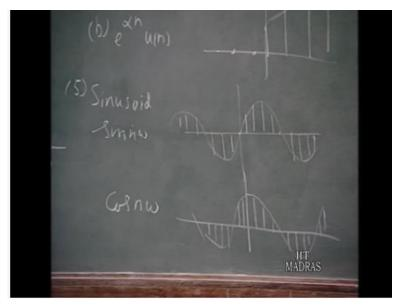
Similarly, you can have a sinusoid you can have sin omega n omega n or n omega which will be in general case this is the envelop the samples will be like this all the samples will fall an envelop which is a sin wave. Similarly, if we have cos n omega it will be a similar situation but this will be now a cosine curve.
