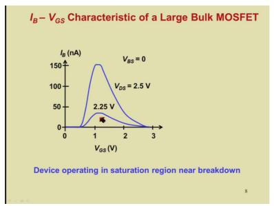
Now let us look at the shape of the IB-VGS curves, which we introduced in the previous module. So the IB-VGS curves are generally plotted for device operating in saturation region
