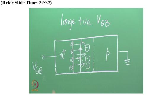
If I consider large positive voltage, then the conditions would be as follows. So here you will have a positive charge on the gate, the positive charge can be created by removing some
