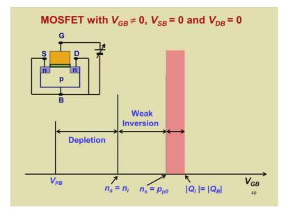
If you increase VGB further, you will encounter a situation where the inversion charge will be equal to the depletion charge. Now let us sketch that here. You increase VGB further, so inversion charge now this in electron concentration will be increased further. It turns out that the depletion charge does not increase much beyond this point. This has been proved by numerical calculations also.
