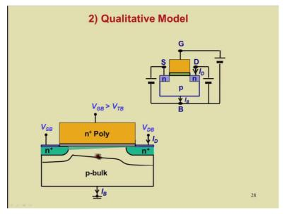
Now let us look into the charge conditions in the MOSFET for the biasing arrangement that we discussed. For gate to bulk voltage more than a value known as a threshold voltage, you have inversion layer of mobile electrons at the interface in an N-channel MOSFET. Beneath the inversion layer, you have a depletion layer from which all carriers are depleted out. Now for sufficiently large value of VGB or VTB, you have a significant current flowing from drain to source if VDB is more than VSB.
