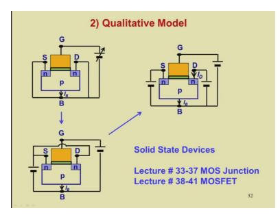
First we analyze the charge conditions in a MOSFET in which only VGB is applied. VSB and VDB are shorted. This is a simple situation. So after this analysis, we move on to analyzing a device in which there are 2 biases VGB and VSB. The VDB = VSB as shown here so drain and source are shorted therefore there is no drain to source current in this case.
