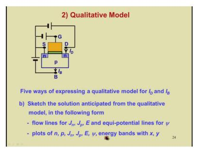
Apart from these 2 ways, the other ways are sketch the solution anticipated from the qualitative model in the following form, flow lines for Jn, Jp, E and equi-potential lines for psi and plots of n, p, Jn, Jp, E, psi and energy bands with x, y that means we must be able to sketch the spatial distribution of carrier concentrations, carrier current densities, electric field, potential and energy bands.
