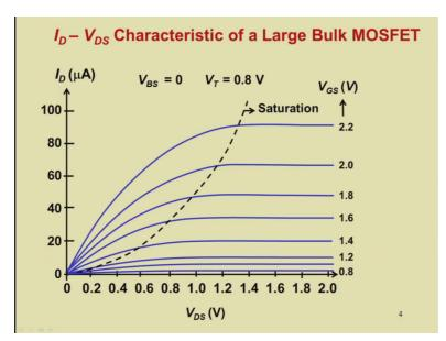
This is a ID-VDS map. The important features here are that the drain current rises as you increase the VDS and progressively the rise tapers off and beyond some point the current becomes almost constant. This is the saturation region. Now the point at which saturation happens are the value of VDS at which the current saturates goes on increasing as VGS increases.
