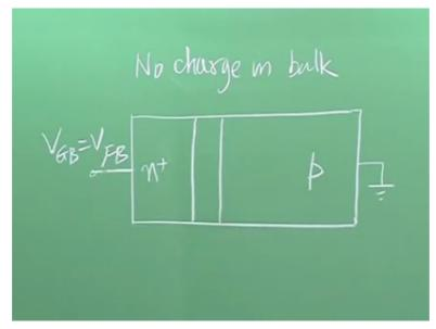
So this is VGB = VFB. So here no charge in bulk or substrate. Now does it mean no charge in the gate? We will come to that point shortly. Let us first talk only about no charge in the substrate. Why should this condition be called flat band okay? For that we have to draw the band diagram in the piece of state for this condition.
