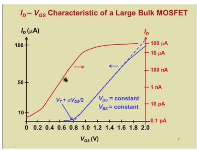
We change the ID axis to a log scale. Here you can see that the ID as a function of VGS is linear when the ID is plotted on the log scale, which means ID-VGS characteristics near VGS = VT that is this region are all exponential in nature ID as the function of VGS is exponential. **(Refer Slide Time: 07:12)**
