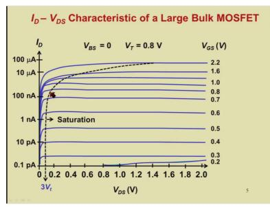
Now when you do that you can see here that the region VGS < VT is expanded a lot. The important feature to be observed here is that the increment in ID on the log scale is uniform for uniform increment in VGS, which means ID versus VGS is exponential for VGS < VT. So this is something we would like to explain. Another feature that you see is that the value of VDS for which the current saturates is approximately constant at 3 times VT for VGS < VT.
