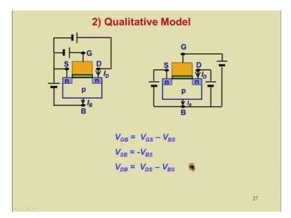
Now let me repeat an important point. In circuit applications, the device is always biased with source as the common terminal. However, from the point of view of device modeling where we want to derive the expression for current as a function of the terminal voltages starting from device physics it proves more convenient to bias the various terminals of the device with respect to the bulk.
