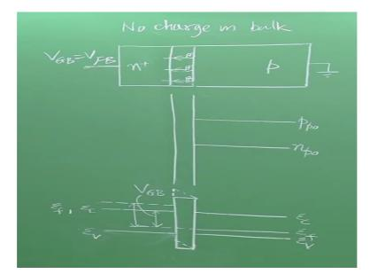
Now before that let us draw the concentration. So if I am going to draw the concentration, if there is no charge that means the hole concentration remains = Pp0 and electron concentration remains = Np0 because the substrate is uniformly doped no charge means that the carrier concentration is constant. Please note, that if this is non-uniformly doped, carrier concentration would not be constant even if there is no charge okay.
