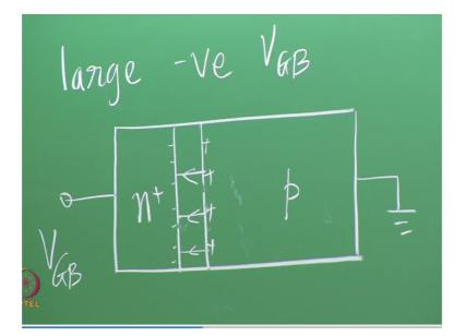
Now we will draw the MOSFET in such a way that your gate terminal is to the left and the bulk is to the right. In other words, as compared to this diagram here, I am going to turn the MOSFET 90 degrees, move this gate to the left so that the bulk comes to the right. The reason for that is we would like to plot various charge-field conditions in the device and those conditions are best plotted with one axis, the spatial axis the distance horizontal.
