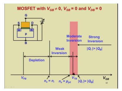
Now this region is called moderate inversion and when QI is more than QB, the range of VGB here is referred to for this range of VGB the device is referred to be in strong inversion because the surface has become strongly n-type as compared to the bulk, which is p-type. In the moderate inversion, you have the voltage called the threshold voltage. Now we are putting a suffix B here because the gate voltage is with respect to bulk.
