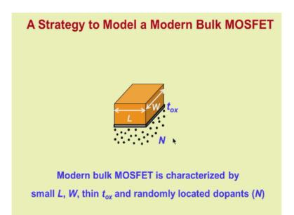
The condition in a modern MOSFET is depicted using this diagram. Note that we are only showing the essential features here and this is a schematic showing the important aspects, which needs to be considered while modelling a modern MOSFET. A modern bulk MOSFET is characterised by small values of L and W, that is the channel length is small and W is also small.
