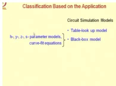
The Black-box model examples of these are h, y, z, or s parameter models or curve-fit equations, here the devices treated as black-box and its terminal are input output characteristics are modelled in terms of a few parameters.
