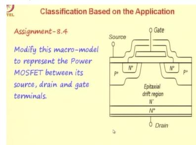
Now modify macro-model that you find in the Wikipedia to represent the power MOSFET between its source, drain and gate terminals, so Wikipedia gives the MOSFET when this N+ is replaced by P+ using that model and using appropriate modification of the model you are expected to represent this power MOSFET structure.
