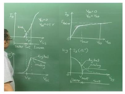
So what is the drive current look at the ID VDS characteristic of a MOSFET, the current corresponding to VDS = VDD that is a maximum current in the device this is called the drive current, the analog model on the other hand both DC and small-signal characteristics such as gd, gm and gmb that is transconductance due to body effect should be predicted accurately, so that is the difference between the goals of the 2 models.
