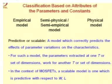
Now let us consider another classification that is based on attributes of the parameters and constants, if all the parameters have no physical meaning or none of the parameters have physical meaning then the model is said to be empirical, on the other hand if all parameters in the model have a physical meaning then it is a physical model, however most models belong to the category of semi physical or semi empirical.
