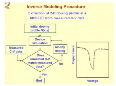
So broadly the flowchart of this activity would be as follows, you assume some initial doping profile and do a device simulation using that doping profile, so the doping profile you should assume initially would be reasonable based on your experience of varies MOSFET, now do a device simulation to get the C-V characteristic for this doping profile.
