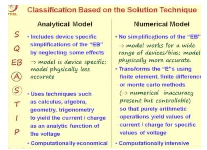
Classification based on the solution technique, you have analytical models and numerical models, so analytical model tends to be device specific and physically less accurate than numerical models which work for a wide range of device or bias conditions, though there is numerically inaccuracy in numerical model because of the method of solution, the inaccuracy can be controlled by increasing the amount of computation.
