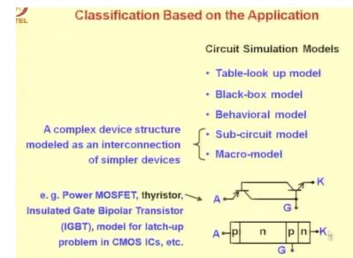
Another class of models is Sub-circuit or Macro-model, a complex device structure modeled as and interconnection of simpler devices, let us look at some examples of these type of models you can look at the internet and find macro-models or sub-circuit models for power MOSFET, thyristor, Insulated Gate Bipolar Transistor and model for latch up problem in CMOS ICs, by way of example we will show here a macro-model of a thyristor.
