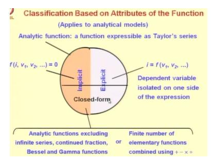
Similarly, another form of classification for analytical model is implicit and explicit closed-form model could be either of implicit variety or the explicit variety, it all depends on how many iterations or how much computations are required to calculate the quantity of interest, if you need infinite number of iterations are extremely large computations to calculate the quantity then the model is not closed-form.
