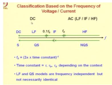
Next we considered classification based on the frequency of voltage or current the classification was DC and AC where AC can be further classified into low frequency, intermediate frequency and high frequency as shown in the diagram, since this is a logarithmic scale of frequencies, the DC or static models can only be represented for f = 0 which will go which will be located at - infinity and that is why this either of these is shown to be extending towards – infinity.
