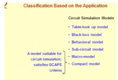
The final type of circuit simulation model and probably the most important type of circuit simulation model is the Compact model, it is the model suitable for circuit simulation which satisfies the GCAPS criteria, in our course we shall be discussing about compact models of devices, so the models which will be derived for MOSFET and any other device would be of the compact variety.
