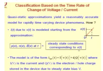
The quasi-static approximations yield a reasonably accurate model for rapidly varying device phenomena, now how do you do that well they get the current instantaneous current as a function of instantaneous voltage starting from the approximation that the distribution of holes, electrons and electric field at any time is approximately = the steady state conditions corresponding to the voltage at that instant of time.
