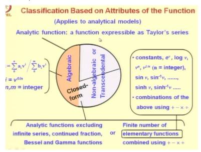
Then we consider classification of models based on attributes of the function, for analytical models we said that the mathematical function could be either algebraic or non-algebraic or transcendental and further it could be closed-form, we explained what is the meaning of algebraic closed-form and non-algebraic or transcendental functions.
