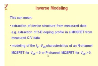
Let us look at the meaning of word Inverse modelling it can mean 2 things, one meaning is extraction of device structure from measured data example extraction of 2-dimensional doping profile in a MOSFET from measured C-V data, another meaning is modeling of the ID VDS characteristic of an N-channel MOSFET for VDS < 0 or P-channel MOSFET for VDS > 0, so normally we will talk about VDS > 0 for n-channel MOSFET so all these curves are for n-channel MOSFET.
