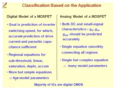
Another classification based on the application we discussed was digital model and analog model, digital model has simple equations and few model parameters, though the number of equations is large they are simple and therefore number of parameters is few, on the other hand the analog model because of the requirements that it must predict the conductance's accurately it has a complex equation though it is a single equation but has many model parameters.
