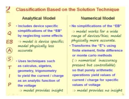
Analytical model provides insight while numerical model provides does not provide insight.
