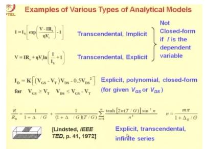
Let us look at examples of various types of analytical models, consider the model of a real diode I = Is exponential V - I time series resistance divided by eta times the thermal voltage -1, the same equation written in a different form with V on one side or the left hand side and the current I on the right hand side, now this form is transcendental and this form too is transcendental because it involves logarithmic functions.
