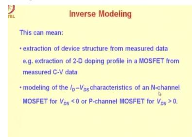
Finally, we talked about inverse modeling which could mean extraction of device structure from measured data or modeling of the ID VDS characteristics of an n-channel MOSFET for VDS < 0 or p-channel MOSFET for VDS > 0.
