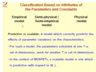
Classification based on attributes of the parameters and constants, so models would be empirical in which case none of the parameters have physical meaning or they could be physical in which case all parameters have physical meaning, most of the models fall in the semi physical or semi empirical model variety however efforts are constantly on to increase the physical content of the model and therefore you talked about making models more predictive or scalable.
