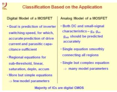
Let us look at a final classification based on application, namely Digital model and Analog model of a MOSFET, digital model the goal is prediction of inverter switching speed for which accurate prediction of drive current and parasitic capacitance is sufficient.
