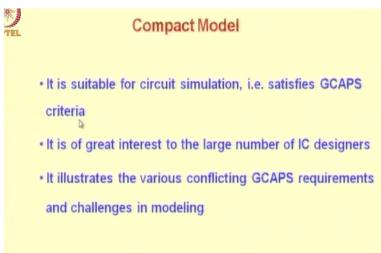
We are going to discuss compact models in this course for various devices and therefore we pointed out a few features of these models it is suitable for circuit simulation that satisfies GCAPS criteria, so here continuity physical basis, in physical basis you have the asymptotic correctness being a very important criterion accuracy, simplicity and generality. The continuity is an important requirement because we discussed the method of solution used.
