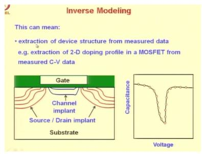
We just let us illustrate quickly how does inverse modeling extract the device structure from measured data, suppose we want to extract these 2 dimensional doping profile of this MOSFET from C-V measurements here is the capacitance versus voltage between the gate and the substrate, now from this data you want to extract this information about the 2 dimensional doping profile.
