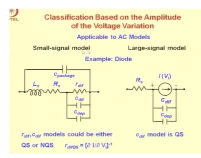
Then we consider classification based on the amplitude of the voltage variation, small-signal models and large-signal models, in large-signal models you have the device represented by a dependent current source, voltage dependent current source where this current I is a function of Vi follows the DC model.
