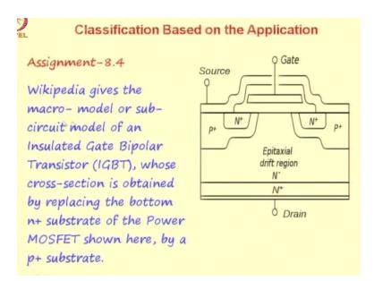
Now here is an assignment related to the macro-model, Wikipedia gives the macro-model or subcircuit model of an Insulated Gate Bipolar Transistor (IGBT) whose cross section is obtained by replacing the bottom n + substrate of the power MOSFET shown here by a p + substrate, this is the structure of a power MOSFET if you replace the N+/P+ this becomes an Insulated Gate Bipolar Transistor.
