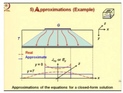
Therefore, let us look at another method which can be used to get a closed form solution. So this is the picture of a spreading resistance this is a cross section view and this is the 3D view. So current flow lines in the cross section are shown here based on this current lines one makes the following approximations about the current flow. So you assume that the current flow expands at a constant angle from the top contact on either side.
