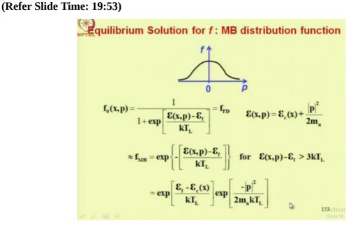
Now from the first level course you know that this particular function is nothing but the Fermi–Dirac function FD. So the Fermi–Dirac function is a solution of the Boltzmann's Transport Equation under equilibrium. However, now how do we get the shape like this? So, normally we use a Maxwell-Boltzmann approximation of this Fermi-Dirac function and if you plot this function it will give you the shape after substituting for E in terms of the potential energy and P square/2Mn.
