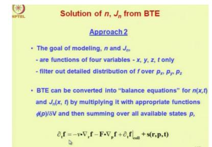
The goal of modeling n and Jn are functions of 4 variables only x, y, z and t and filter out detail distributions of f over Px, Py and Pz. So, in the process of finding out n and Jn from f we are filtering out the effects of Px, Py and Pz. You know that from formula for the equations of n and Jn. Now that being the case, why not adopt this approach. The BTE can be converted into balance equations for carrier concentration n and current density Jn
