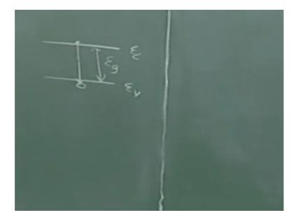
So this is the diagram, Ec Ev and this the recombination, right, process in which the electron jumps into a hole and this energy gap. So, this energy that is released. Now let us show the correspondence of this equation with the whole continuity equation. Now here we are writing the term G - R because the net generation or recombination for holes and electrons would be equal because the processes are always balanced, right?
