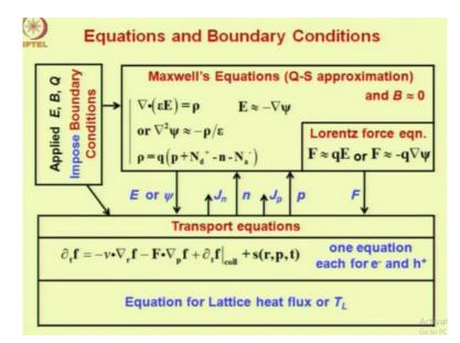
So, here you have the Maxwell's equations with Quasi-static approximation and magnetic field = 0. There are 2 equations E = - grad psi equation and then you have Lorentz force equation which gives you the force because of electric field or potential gradient. Now this force and the electric field that is given here is used in the Boltzmann transport equation to solve for the distribution function f.
