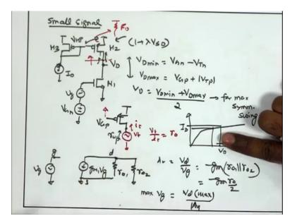
So, once again if I go back to my small signal model and I try to see what is the small signal resistant between the drain node that is this output node and the AC ground that is once again just going to be parallel combination of r o 1 and r o 2.
