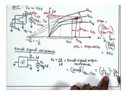
So, if you recall our discussion we were talking about the small signal model where we are applying some six small signal voltage at the drain of the MOSFET and trying to see what is the resulting small signal current.
