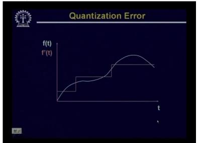
you will find that in this, the green curve, it shows the original input signal and this red staircase lines, staircase functions it shows that what is the quantization signal, quantized signal or f hat, f prime t.
