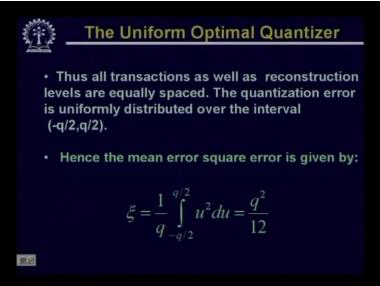
quantization error in this case is uniformly distributed over the interval minus q by 2 to q by 2. And the mean square error in this particular case if you compute will be given by 1 upon q u square d u you take the integral from minus q by 2 to q by 2 which will be nothing but q square by 12.
