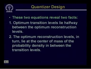
the optimum reconstruction levels in turn lie at the center of mass of the probability density in between the transition levels. So which is given by the second equation
