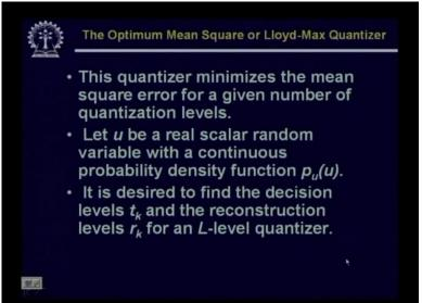
So for quantizer design the aim of the quantizer design will be to minimize this quantization error. So accordingly we have to have an optimum quantizer and this Optimum Mean Square Error quantizer known as Lloyd-Max Quantizer, this minimizes the mean square error for a given a given number of quantization levels.
