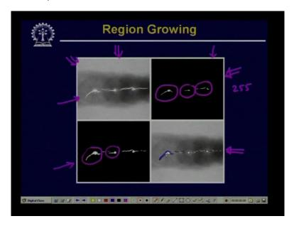
So, here is an example, this is the x-ray image taken from a weld. And you find that, in case of this x-ray image, there may be some cracks within the welded region or there may be some faults within the welded region, and these faults can be captured by using x-ray image.
