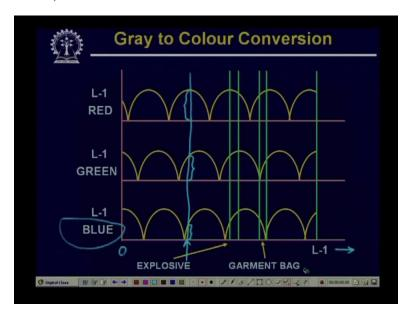
The transformation functions are usually a sinusoidal functions. So here what you have is you have this is the red transformations, this is the Intensity values along the horizontal axis, we have the Intensity values of grey scale image, which is varies from zero to the maximum value N minus 1.
