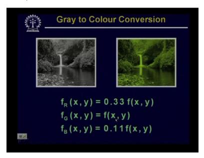
Whereas in this particular case our Pseudo coloured image appears to be green because here F (x,y) F the green component, the green plane is same as F (x,y) whereas red and blue are taken as scaled down version of F (x,y). So if we change the weightage of this a different function of this different red and blue green, red and blue planes. The colour appearance will again be different.
