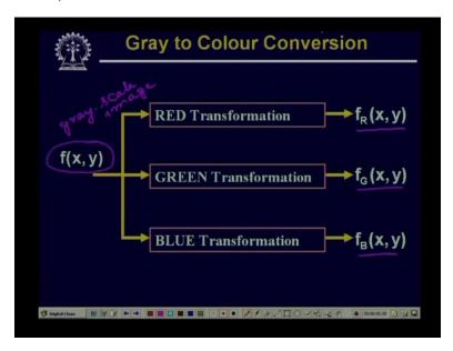
So here what we have shown is to different Intensity intervals we have assigned different colours. Now when we go for grayscale to colour transformation then what we have to do is, if I have an Intensity image or grayscale image that corresponds to a single plane, I have to convert that to three different planes that is R G B red, green and blue planes and those red, green and blue planes when they combine together there combine together they give you an interpretation of a colour image.
