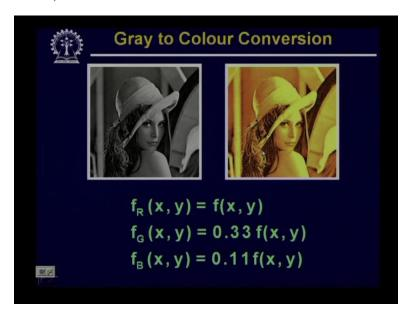
In our earlier case, the coloured image was showing more of red component because in this case, FR was as seen as F(x,y) whereas green and blue where scale down version of F(x,y).
