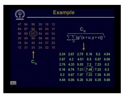
So if I do that normalization this is my original cross correlation coefficient matrix that I have computed earlier, and by using the normalization what I get is the normalization normalized cross correlation coefficient matrix which comes like this.
