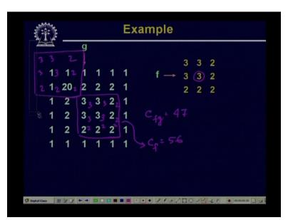
Say here this is the image g which is given in the form of a 2 dimensional matrix. 2 dimensional array of size 6 by 6 and our template is of 3 by 3 matrix which is given on the right hand side, ok. Now, if I calculate the Cfg for this, so what I have to do is, to find out the match location, I have to take the template, shift it all possible location in the given image g and find out the cross correlation or the similarity measure at that for that particular shift.
