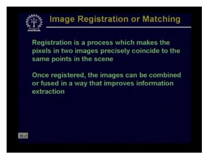
So by image registration what we mean is that the registration is a process which makes the pixels in two images precisely coincide to the same points in the scene. So by registration what you mean is, if we are having two images of the same scene, may be the images, two or images are acquired with different sensor located at different positions or maybe the images are acquired using the same sensor but at different time instance at different instant of time.
