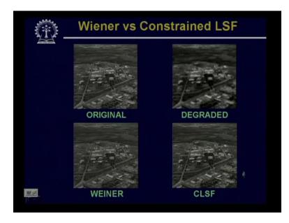
Now using this kind of approach, what we have obtained is we have got some reconstructed image. So here you find that it is the same original image this is the degraded version of that image. On the bottom row the left hand side gives you the reconstructed image using the wiener fettering. And again on the bottom row on the right hand side this gives you the reconstructed image which is obtained using the constrained least square filter.
