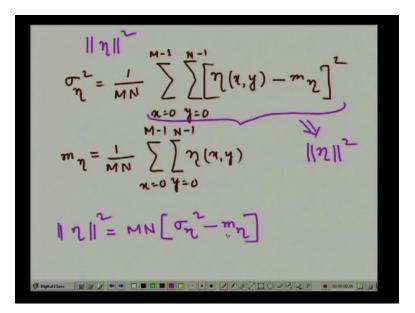
So we can obtained the noise estimate or we can compute the noise term that is eta square in our expression which is used for this constrained least square filtering in this way. We have the noise variance which is given by sigma n square sigma eta square which is nothing but M into N into double summation eta (x,y) minus M eta. Which is the mean of the noise square where y varies from 0 to N-1 and x varies from 0 to M-1.
