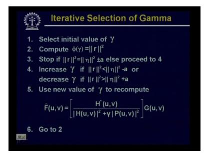
Now given this background an iterative approach, iterative algorithm for estimation of the value of gamma can be put like this. So you select an initial value of gamma then compute y phi gamma which is nothing but Euclidean norm of r, then you terminate the algorithm if r square is equal to n square, here it has been written as eta square plus minus A.
