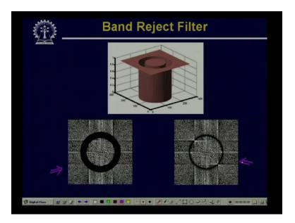
So this is the perspective plot of an ideal band reject filter and here the band reject filter are shown super imposed on the frequency plane. So on the left what I have is an ideal band reject filter and on the right what I have is the corresponding Butterworth band reject filter. So by using this band reject filter we are removing a band of frequencies from the Fourier coefficient corresponding to the frequency of the noise.
