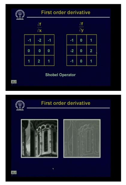
So for computing the first order derivative along x direction, the left hand side shows the mask and for computing the first order derivative along y direction, the right hand side shows the mask, and later on we will see that these operators are known as Shobel operators.
