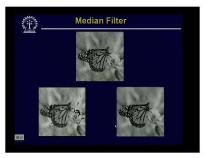
Then, this shows another median filter output result uhh the bottom two images on the left side it is the image obtained using the box filter, on the right hand side it is the image obtained using the median filter. The enhancement using the median filter over the box filter is quite obvious from this particular image.
