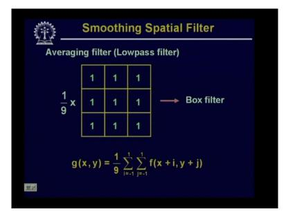
So let us first quickly see that what we have done in the last class. So in the last class we have talked about the averaging filters or low pass filters and we have talked about two types of spatial masks which are used for this averaging operation.
