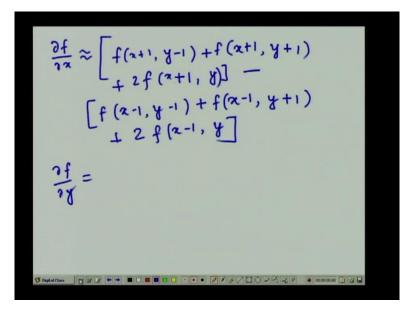
So this is what gives us the first order derivative operator on an image, and if I want to obtain del f del x, you find that this del f del x can simply be computed as [f(x+1), (y - 1)+f(x+1,y+1)+2f(x+1,y)] - [f(x -1, y -1)+f(x -1,y+1)+2f(x -1,y)]. So this is the first order derivative along x direction and in the same manner we can also obtain the first order derivative in the y direction.
