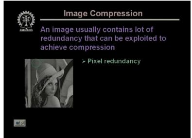
So whenever we talk about an image, the image usually shows 3 kinds of redundancies. The first kind of redundancy is called a pixel redundancy which is just shown here.
