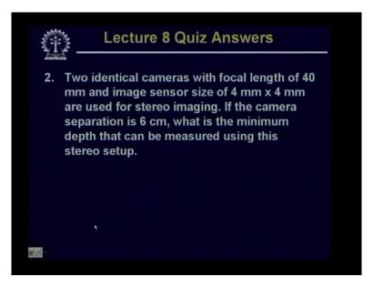
Second question was to find out what is the minimum depth that can be obtained by using the stereo camera where the the geometry of the stereo camera was specified.
