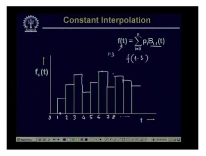
As, we have said earlier that using these B-Splines a function is approximated as f(t) equal to piBi,1(t) or Bi,k(t) where i varies from 0 to n. So, in this case let us take the value of k to be equal to 1 that means we have a B-Spline of order 1. And we have shown that if we have a B-Spline of order 1 then the nature of the B-Spline function is it is constant between i and i+1 and which is equal to 1.
