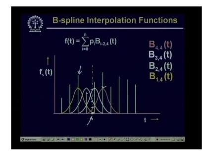
And by using this now the interpolation can be obtained by as if I go for cubic interpolation that f(t) is equal to piBi-2,4(t), where the summation has to be taken from i equal to 0 to i equal to n. And, here it gives that if I want to interpolate this function at this particular point, the weight given by this particular sample is only this much, the weight given by this particular sample is this much, the weight given by this particular sample is weighted by this much.
