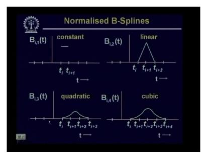
Now, after giving these equations let us try to see that what is the nature of this of this B-Spline functions. So we find that Bi,1(t) because it will be equal to 1 for i equal to 1 to 2, between i equal to 1 to 2, this Bi,1(t) will be equal to constant and it will be equal to 1. So, this first figure in this particular case tells you that what is the nature of this B1 Bi,1.
