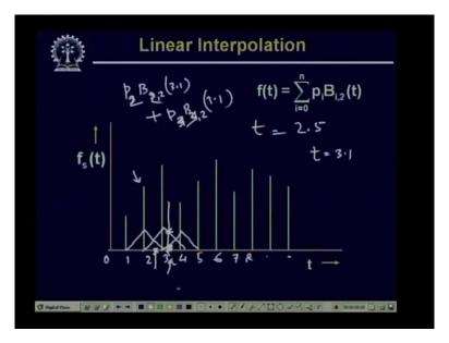
Similarly, between t equal to 2 and t equal to 3 the interpolated values is equal to fs,2 and so on. Similarly, if I go for interpolation using say linear interpolation where value of k is equal to 2 in that case again you find that if I put say t equal to 0 here, t equal to 1, t equal to 2, t equal to 3, 4, 5, 6, 7, 8, like this now B1,2 is a linear function between 1 and 3. So B1,2 is something like this. Similarly, B2,2 is something like this, B3,2 is something like this.
