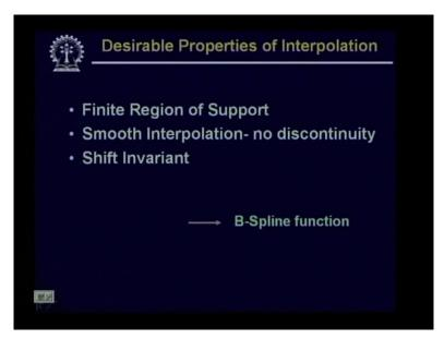
The second desirable property is the interpolation should be very smooth that is the interpolation should not introduce any discontinuity in the signal. And the third operation is the interpolation should be shifting variant, so if the signal is shifted or given some translation then also the same interpolation function should be available should be done. And the B-Spline function is one such function which which satisfies all these three desired properties.
