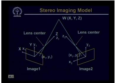
w in the three-dimensional world, three-dimensional space you find that the corresponding image point in image 1 is given by x 1 y 1 and the image point for the same point w in image 2 is given by x 2 y 2. I assume that both the cameras are identical that means they have the same value of wavelength lambda so they will have the same perspective transformation as well as
