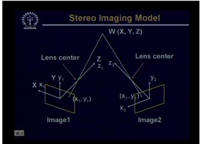
inverse perspective transformation I also get equation of another straight line on which this equation of w will exist. So now you find that by using these two images I got equations of two straight lines. So if I solve these two equations, then the point of intersection of these two straight lines gives me the x y z coordinate of
