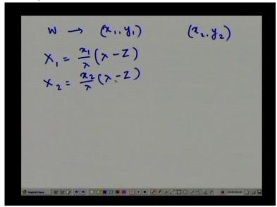
where this capital X 1 is the x coordinate of the point w with respect to the camera coordinate of camera 1, and capital X 2 is the x coordinate of the 3D point w with respect to
