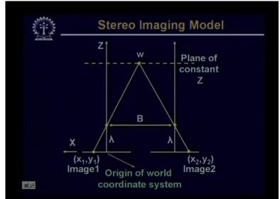
as a setup where find that this x y plane of both the cameras are now perpendicular to the plane So I have x axis which is horizontal, the z axis which is vertical and the y axis which is perpendicular to this plane So in this figure I assume that the camera coordinate system of one of the cameras, in this case the camera 1 which is also called the left camera is aligned with the 3D world coordinate system
