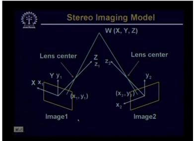
where on the left side I have image 1, on the right side I have image 2. The image 1 is taken, captured with the help of one camera; image 2 is taken with the help of another camera. So image 1 has the coordinate system say x 1 y 1 z 1. Image 2 has the coordinate system x 2 y 2 z 2. And we can assume that the 3D world coordinate system that is capital X capital Y capital Z is aligned
