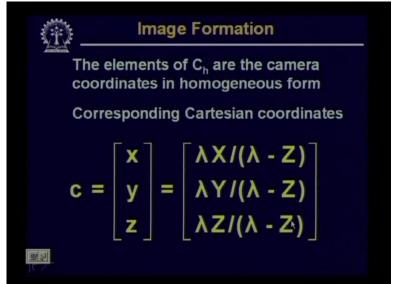
camera coordinate to the Cartesian camera coordinate I find that the Cartesian camera coordinate is given by c equal to small x, small y, small z which is nothing but lambda x divided by lambda minus z, lambda y divided by lambda minus z and lambda z divided by lambda minus z. So, on the right hand side this x, y and z they are all in upper case indicating those are the coordinates of the world point.
