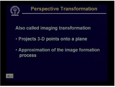
imaging transformation And the purpose of this imaging transformation is to project a 3D point, a 3D world point into an image plane. And this gives an approximation to the image formation process which is actually followed
