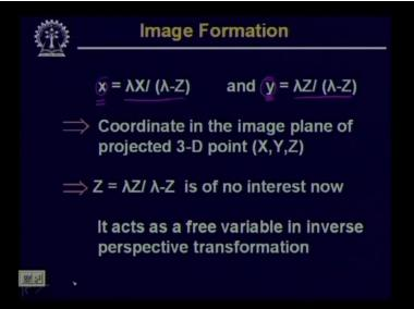
the value of z which is not of importance in our case because in the camera coordinate the value of z is always equal to 0 because we are assuming that
