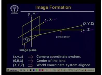
in 3D so this is the point x, y, z in three-dimension and I assume that the center of the lens is at the location 0, 0, lambda. So obviously the lambda which is the z coordinate of the lens
