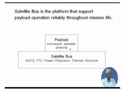
So, let us go back to that old diagram that is satellite bus is the platform that support payload operation reliably throughout the mission life and payload will be microwave repeater and the antenna and the satellite bus is AOCS, TTC, power, propulsion, thermal and structure. Briefly we have gone through each of them except the propulsion within much we have taken its part of AOCS.
