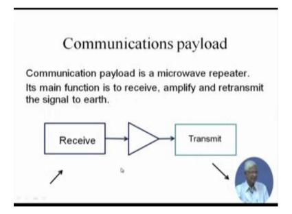
So, now let us concentrate to find out what is there in this payload. Communication payload, what is that? Communication payload we were using from the beginning. The term is a microwave repeater. Its main function then should be to receive, amplify and transmit the signal to the earth and earth was the service area. It receives the signal from the service area, amplify the signal and transmit that. That is what payload is.
