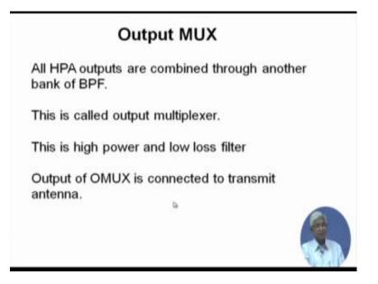
Then, each of these amplifiers output has to be combined again. So, we call another multiplexer which is output multiplexer or which outputs are combined through another band of band pass filter. This is called output multiplexer. These band pass filters are difficult to design because it has to handle high power. They have already power amplifier has been put, this is high power and low loss filter and output mux or OMUX is connected to the transmit antenna.
