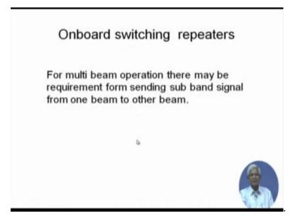
Now, this what you described as a simple conversion of the frequency is called bent pipe or transparent transponder, but in some cases move complex transponders I used which is having on board switching capacity. We will start discussion on this in the next class, right.
