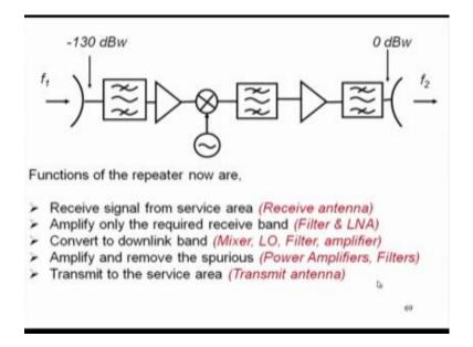
Let us go back to the payload. So, we have minus 130 dBw. Obviously, we have put lot of filters amplifiers and we have to change the frequencies. So, we have to have mixer and down link frequency is lower which is f2 is lower than f1. So, it is down converted again filter, again amplifier and you put and see lot of filter coming. So, each of them can be put into different sub systems.
