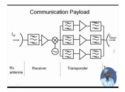
I can draw the picture. Now is the uplink frequency which is coming as it is see antenna and then the receiver is nothing, but the input filter and then, known has amplifier and then down converter. Of course, there is a filter here and after the down converter at that input mux which is de-muxing actually taking place and then amplifiers. I have shown one amplifier and then, output mux which is combined called transponder and then, the transmit antenna which is going as a down link.
