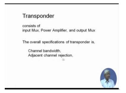
So, a transponder consists of input mux, the power amplifier and output mux and the overall specification of the transponder is channel band width adjacent channel rejection group delay.
