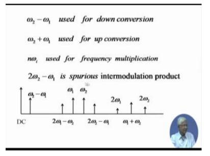
Let us see the advantages and try to find out. So, if there are two frequencies omega 1 and omega 2 in the frequency plot and if you are d c, something will be generated. Omega 2 minus omega 1 will be generated very near to d c and then, 2 omega 1 minus omega 2 and 2 omega 2 minus omega 1 generated near to omega 1 and omega 2. It is two fundamental, 2 omega 1 and 2 omega 2 will be generated far away and then, there will be true only omega 1 plus omega 2 another carrier one.
