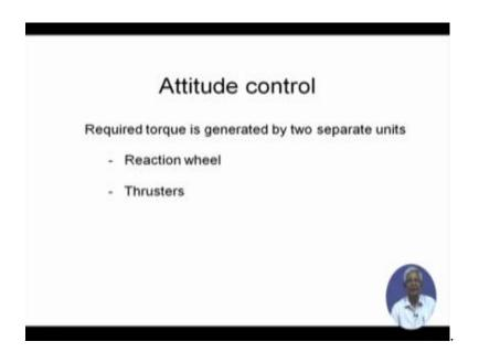
Now, with this you have to do certain control you have sensed it. Now if the sensed information has gone to ground or on board is compared and then a decision has to be taken that you have to control it now how we control it. So, attitude is controlled. There are two types of unit for control one is called Reaction wheel another is called Thrusters.
