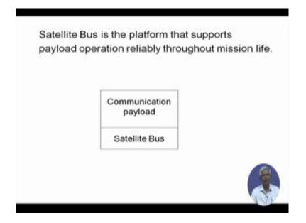
Now, in the Satellite bus it is the bus which carries the payload. So, basically our requirements are the communication payload. The payload can be remote sensing can be meteorology can be scientific in our case it is a Communication payload earlier we used to called we have called it a repeater a microwave repeater. So, let us see what is this bus which carried this payload.
