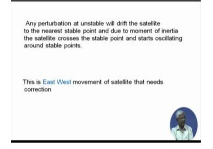
So, any perturbation at unstable point will drift it towards the stable point and oscillator on it due to inertia. These movements are on the equatorial plane. So, it is called East West movement of the satellite that has to be corrected keep it in the position.
