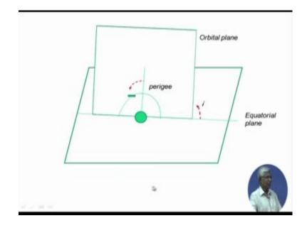
This is the, let say, this is the earth and this is the equatorial plane and for generalization let us say that satellite is Orbiting in a different plane than the equatorial plane and that Orbital plane is making a intimation with the equatorial plane is the perigee and then may be apogee below.
