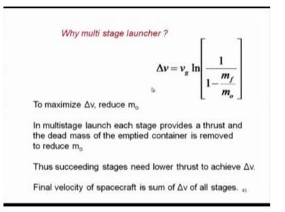
To maximize the delta v we reduce m 0 in multistage launch each stage provides a thrust and the dead mass of the emptied container is removed to reduce m 0. Thus succeeding stages need the lower thrust to achieve delta v and the final velocity some of all the stages of delta v what we get is the multi stage now.
