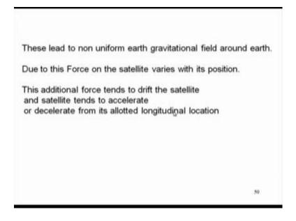
So, therefore, it leads to non uniform earth gravitational field around the earth and due to this force on the satellite varies on its satellite position. So, this additional force trend to drift the satellite from the intended location and either accelerate or decelerate.
