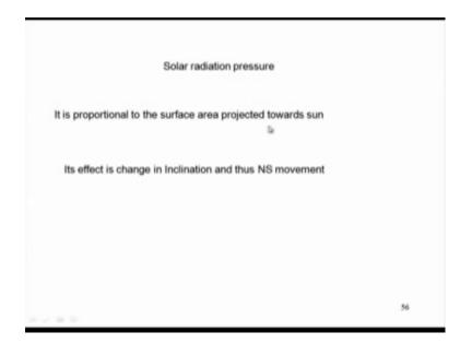
There is the solar radiation pressure which is proportional to the surface area projected towards the sun its effect also in make the non (Refer Time: 27:01).
