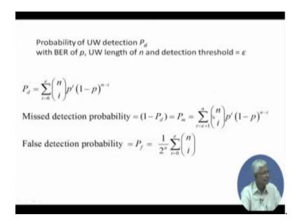
Now this probability of detection is you know this type of expression probability of detection o for with the error tolerable error is I equal to 0 to epsilon n c I small p is bit error a probability and small m is the length of the unique word. So, I minus p to the power of n minus I and error threshold is epsilon.
