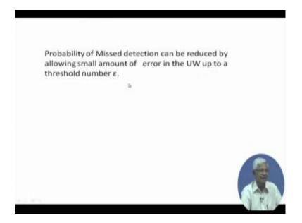
So, compare bits within the time window only and window repeats at the frame rate probability of missed detection can be reduced by that is probability of false detection reaction by aperture technique and probability of missed detection can be reduced that, if there is a error I tolerate that error. So, I allow some amount of error in the unique word up to a threshold let us say epsilon.
