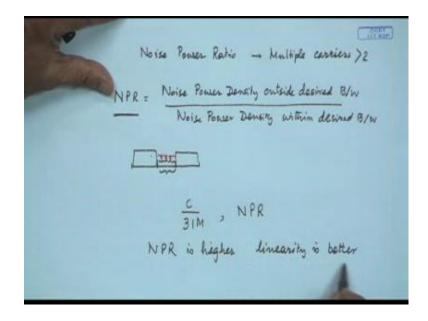
They use a term called noise power ratio, this is for multiple carriers that is greater than 2. And this NPR is defined as noise power density; that noise power which is generated due to multiple carriers is going to fall at once place so that is called desired bandwidth. So, it is noise power density outside desired bandwidth divided by noise power density within desired bandwidth; is very simple.
