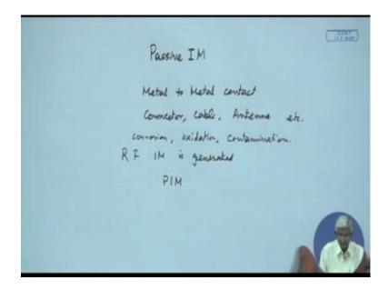
There is one more thing that people come across that is called passive inter mod product, this is a not by active device. When there is a metal to metal connect like in connector, cable, input to the antenna, etcetera. Due to corrosion, oxidation, contamination that RF inter mod is generated. Because of these things it creates a non-linearity in the metal or the conductor which is which is carrying the Rf.
