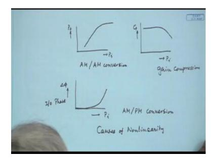
So, let us see that three effects we have seen that is we have seen that power in to power out in dB, the curve goes like this linear and then non-linear; so this one is termed as AM to AM conversion. Similarly, we have seen there is a gain compression, if there is a gain this said and power in this side initially there is a constant gain then gain will start falling when (Refer Time: 21:12) point coming and beyond that.
