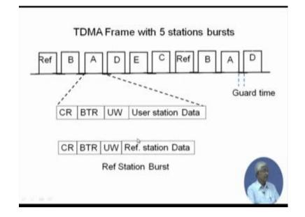
So, these are given certain extra times which are required the you can see in a satellite there is on another transponder, if it is continuously looked you can see that the TDMA frame with five different station A, B, C, D, E is shown here there is a reference bursts and then say first burst time is given to station B second one for station A and then D and E and C like that, and it repeats after.
