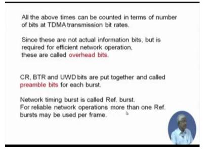
Let just look at it the above times can be counted in terms of number of bits in TDMA transmission bit rate, since these are not actually information bits that is required for efficient operation of the network these are called overhead bits.
