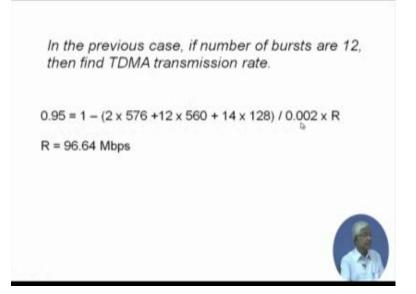
Let us see if the number bursts are 12 and then what is the transmission rate you can find out efficiency is known 12 bits and then frame time is given. So, you can find out that any number is missing you can find out those.
