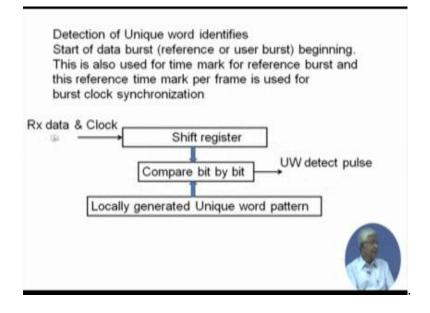
Now, this is the network synchronization part and, but in all these process you have to detect the unique word, which tells you where the data burst start or reference burst data starts. So, detection of the unique word is very important unique word is beginning of a burst. Where they actually data is there this is also used to time mark for the reference burst and this reference burst time mark per frame is used for burst clock synchronization.
