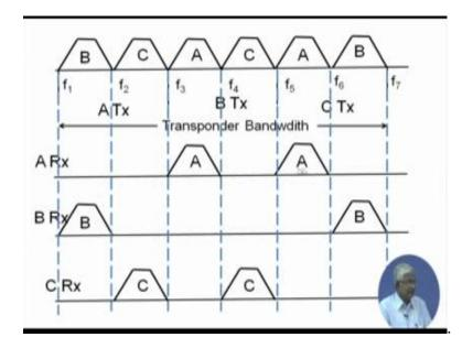
Let us give a quick example pictorially. It is easy, you can realize that let us say there are three stations and three stations are given at two frequency bands each a station A has f 1 f 2 and put a center frequency, but it is total bandwidth. Then B f 3 and f 4 center frequencies. And C f 5 and f 6 center frequencies and with certain bandwidth available here again it is shown that bandwidths are written that is at the transponder.
