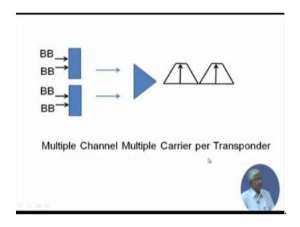
It is possible that multiple channel in multiple carrier also there. So there could be two carriers two separate operators are sharing one transponder and each of them is transmitting multiplex signal could be TV or voice or sound or anything. In this case the transponder is carrying two carriers and both the carriers are multiplex so it is Multiple Channel Multiple Carrier per Transponder. It is some form of definitions.
