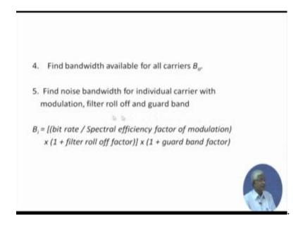
And bandwidth wise that is power wise. Bandwidth wise is also easy find the bandwidth available for all carriers that is total bandwidth supported by the transponder in full transponder case. Then find the noise bandwidth of the individual carrier with the modulation, filter roll off guard band etcetera.
