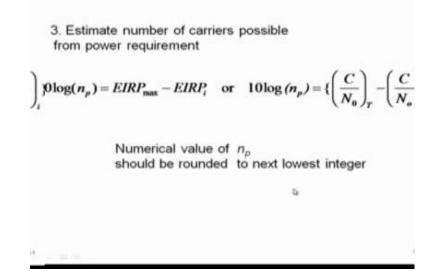
So, estimate the number of carriers possible from the power requirement point of view. It is very simple that the number is the dB subtraction log of the number is dB subtraction of the maximum EIRP satellite can support and individual carrier. And we have assume that all carriers are same, so it is just subtraction of that or in terms of C by N if you do C by N naught total minus C by N naught individual and that will be their log n p.
