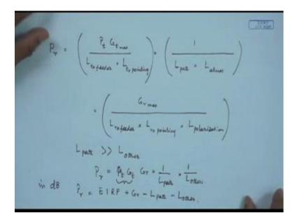
With all this losses then that can be group together and let us see how the expression then becomes. We have Pr which is equal to EIRP Pt into Gt and at the transmit side we have loss due to transmit feeder then loss due to transmit antenna pointing, and then we have the medium which is coming between and the medium there is the path distance so there is a loss due to path. Then loss due to atmosphere, and then we have the receiver where the receive antenna comes into picture.
