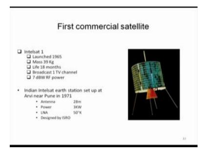
Even with that first commercial satellite, it is called Intelsat 1 was launched in 1965; it has a mass of only nearly 40 kg about; one and half year life time. It could broadcast one TV; analog TV channel and the transmit RF power was 7 dBW RF power, mark dBW this is a power unit in db. When you know convert into direct ratio power, it is equal to 5 watts, this db unit has to be learnt quickly because we will be using it very frequently later.
