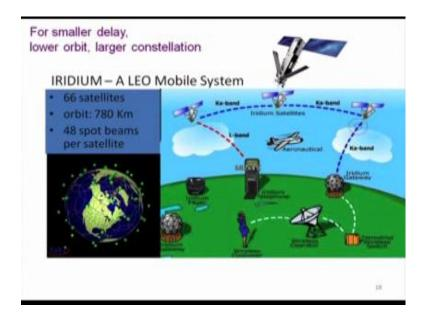
So, such big technologies are there if an much lower of the orbit it is called LEO, 66 satellite constellation was launched by IRIDIUM consortium and each satellite has 48 spot beams anywhere in the world you can communicate via this satellite.
