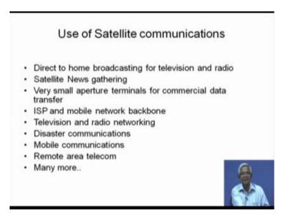
Now, satellite communication can used for direct to home broadcasting to television radios or news gathering, very small aperture terminal, internet service provider and mobile network backbone, television, radio networking, disaster communication, mobile communication, remote area communication lot of things.
