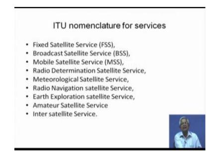
So these terms what I am using is listed by ITU nomenclature on Fixed Satellite Service; FSS, Broadcast Satellite Service; BSS, Mobile Satellite Service; MSS like that there is a big list of that, so these are the terminologies we will be using frequently.
