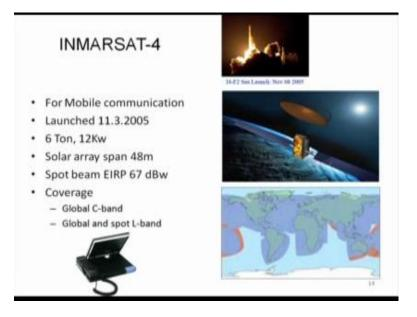
Similarly over the sea, INMARSAT is there, so which is launched in 2005; this is INMARSAT 4, it is 6 ton, 12 kilo watt satellite. It has a solar array of 40 meters, (Refer Time: 15:28) 7 spot beams, these are taken from internet.
