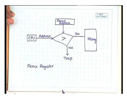
While execution of a user program, the CPU generates the address. The address of the memory location that is to be accessed while execution of the user program. I also have a fence address which is the boundary between the user area and the monitor area. So I have to compare this fence address with the address that is generated by the CPU. So I have to compare these two addresses.
