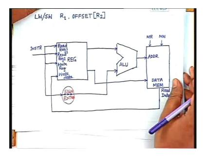
In case of load or store instruction, first input to the ALU comes from the register bank whereas the second input comes from the instruction offset. In case of branch on equal instructions, second input also comes from the register bank that is there are two sources from which the second input to the ALU will come. So I have to multiplex those two sources.
