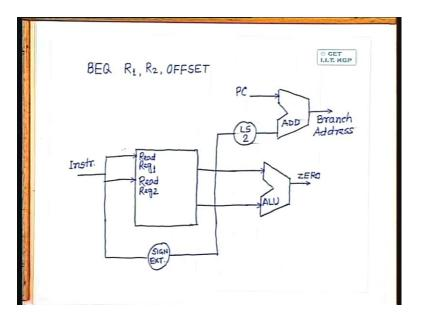
So this left shifted offset is to be added with the current program counter value. So I need an adder unit here. Here what I get is the program counter and this output, this is a simple adder unit. This output gives me the branch address.
