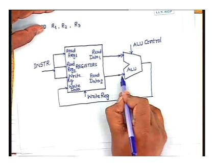
In case of ADD instruction, the second input to the ALU comes directly from the register bank. First input also comes directly from the register bank.
