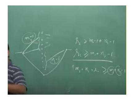
So this is actually setting up the calls where this m1-1 this guys actually using this n3-1, m and if my number of middle stage switches has one more than that so this free and this free thing can be used these free input and output ports can be route can it be actually a call can be set a bit in them using this free middle stage switches, is a worst case occupied switches. So I am not worried about how the others output side is been connected.
