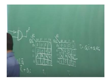
So all toggle T1 and T0 both have to be 00. So I require two of them, so one is for P1 other one is P0, so I have to put a 0 here a 0 because there is no toggling required okay, when it is 01 then also no toggling is required. So here I have to put a 0, when it is 11 no toggling is required. So I have to put a 0 here okay, and when it is 10 then it should go from OFF to intermediate state okay, so Q1 has to be toggled. So it is 00 RC is 10.
