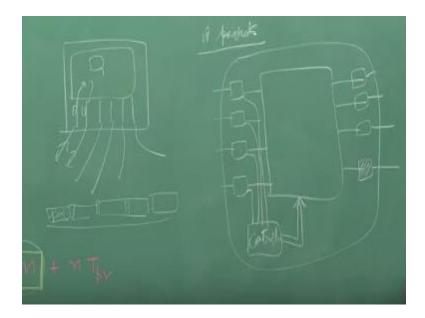
Now these interface boards also has another important function, so that i can handle the variable length packets i will come to that so I am just drawing the four by four these are interface boards this is a cross bar, and I will actually have one control line through which I will get all header information, controller will get and then it will exact row column and control, on this cross bar set up the things.
